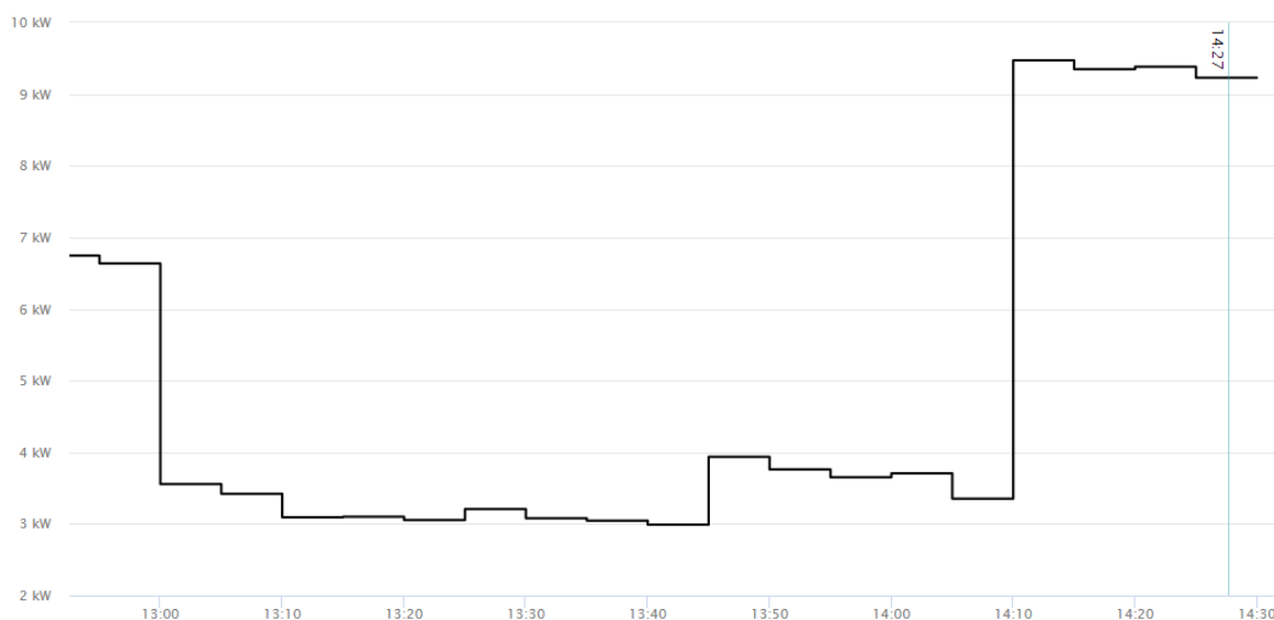
Real-time power metering from the charging point during testing
